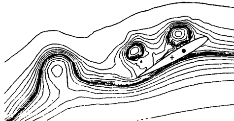
Figure 9. Time evolution of the flow structure; Re = 10000 , f^* = 0.5 , \alpha = 30^\circ , \Delta\alpha = -7^\circ , \xi_\infty = 0.72324
